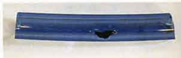
Burned material is discharged into the product wall creating a material defect.
